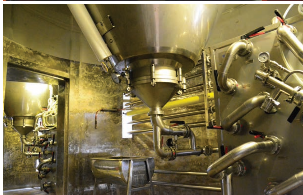
The sensory analysis room (top) and bottom cone and diverter panel of an outdoor tank (bottom) at Firestone Walker Brewing Company
